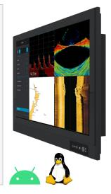
In addition there are options such as factory mounted Projected Capacitive Touch Screen (Multitouch, USB interface), Optical Bonding, variations of CPU, Storage Devices, operating systems and prepared for WiFi and Bluetooth antennas. By factory default the unit is ECDIS Compliant.
