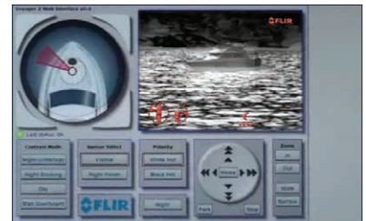
Select FLIR thermal imagers feature IP addressability that provides remote internet access so crews can operate the camera from any location with an internet connection, even when they're not on board.
